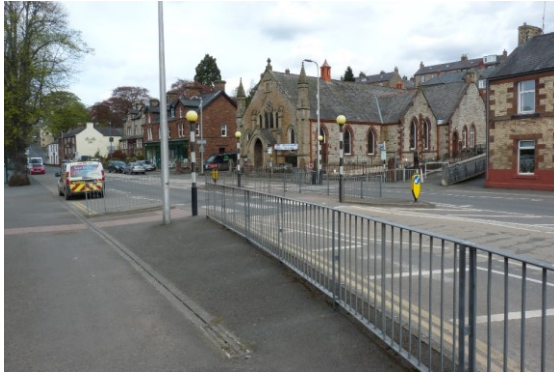
Figure 86 Pedestrian crossing with guardrails
